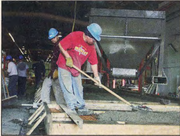
MEN AT WORK: Smith-Midland workers, left, spread concrete for sound walls at the company's Midland plant. Will Guevera, center, adds the finishing touch. Quinton Noakes, right, works the controls of the cement mixer.
