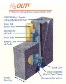
caulk joint, secondary drainage, streetlevel leak detection system. Caulk leaks exit to the outside of the building and can be located within 20 feet of the leak whether the building is five days, five years or 20 years old, says the company.
